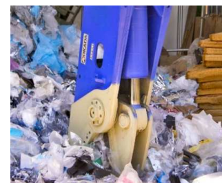
Some machinery treats soft waste such as wood waste, plastic waste, and tires
